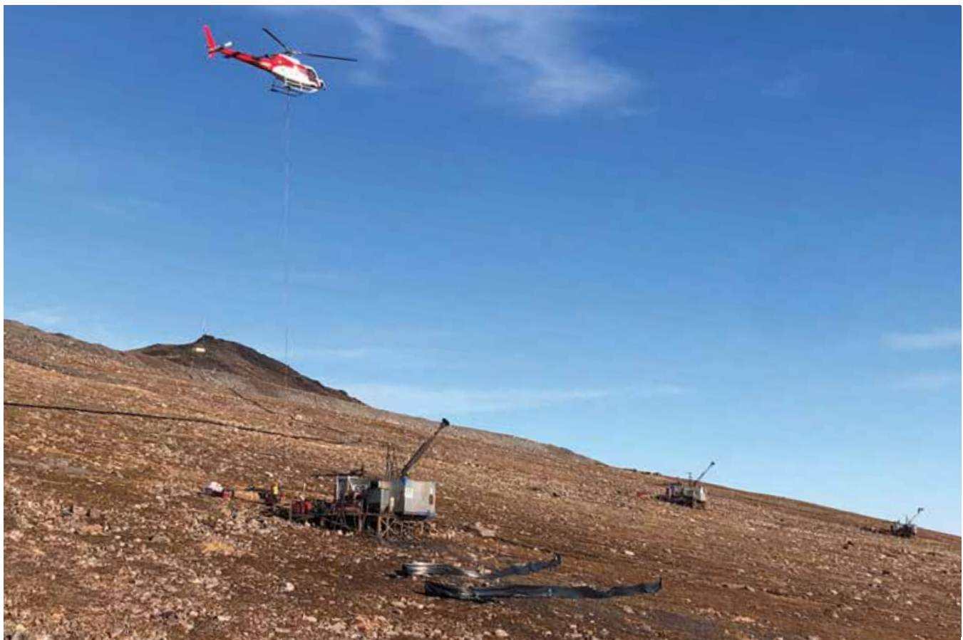
Exploration drilling on the North Limb zone of Deposit No. 1 at the Mary River mine, northern Baffin Island. Courtesy of Baffinland Iron Mines Corp.
