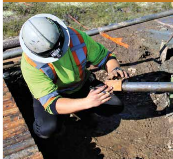
A driller orients a core sample from the Ulu gold project. Courtesy of Blue Star Gold Corp.
