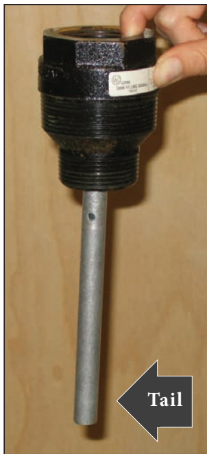
4.9a Heating oil tank vent whistle: the tail of the vent whistle protrudes into the oil tank; the vent pipe screws into the top of the vent whistle.
