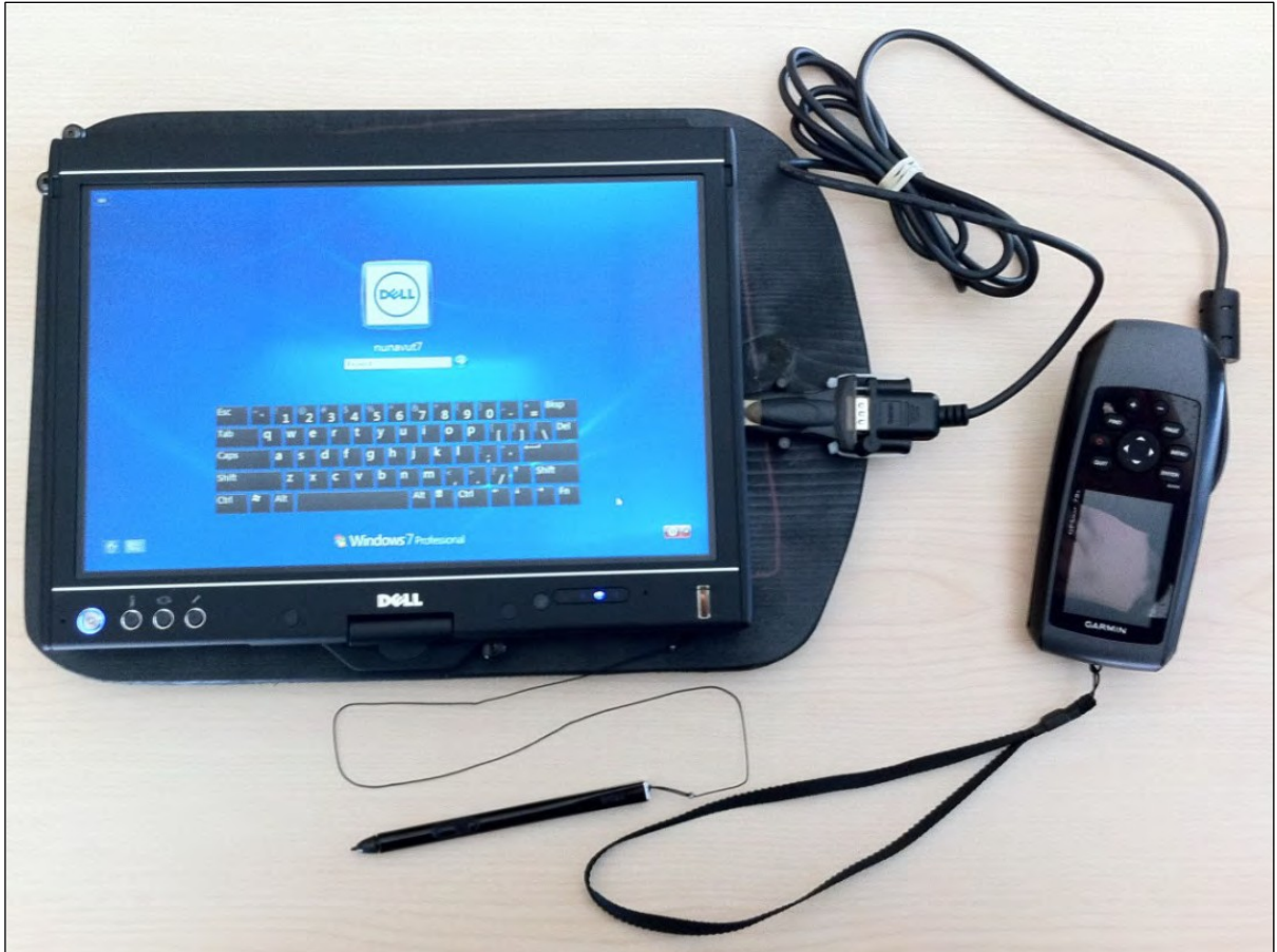
Figure 9 Hardware components of the Aerial Wildlife Survey - Observation Collector (AWS-OC) software and illustration of the Garmin GPSmap 78s cable setup.
