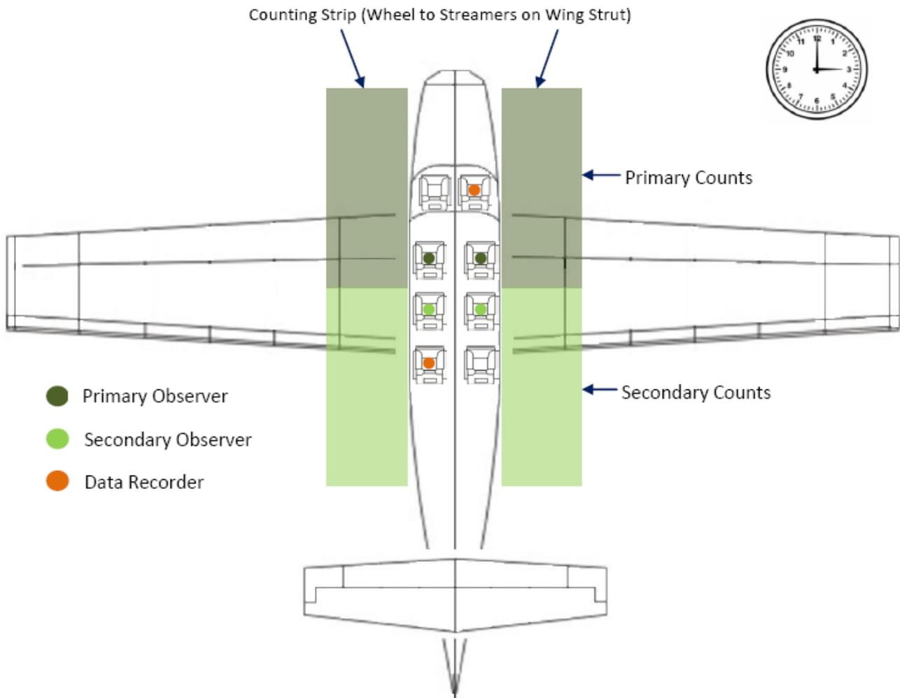
Figure 8. Observer position for the double observer pair method employed on this survey. The secondary observer calls caribou not seen by the primary observer after the caribou have passed the main field of vision of the primary observer. The small hand on a clock is used to reference relative locations of caribou groups (e.g. "Caribou group at 3 o'clock" would suggest a caribou group 90° to the right of the aircraft's longitudinal axis.).
