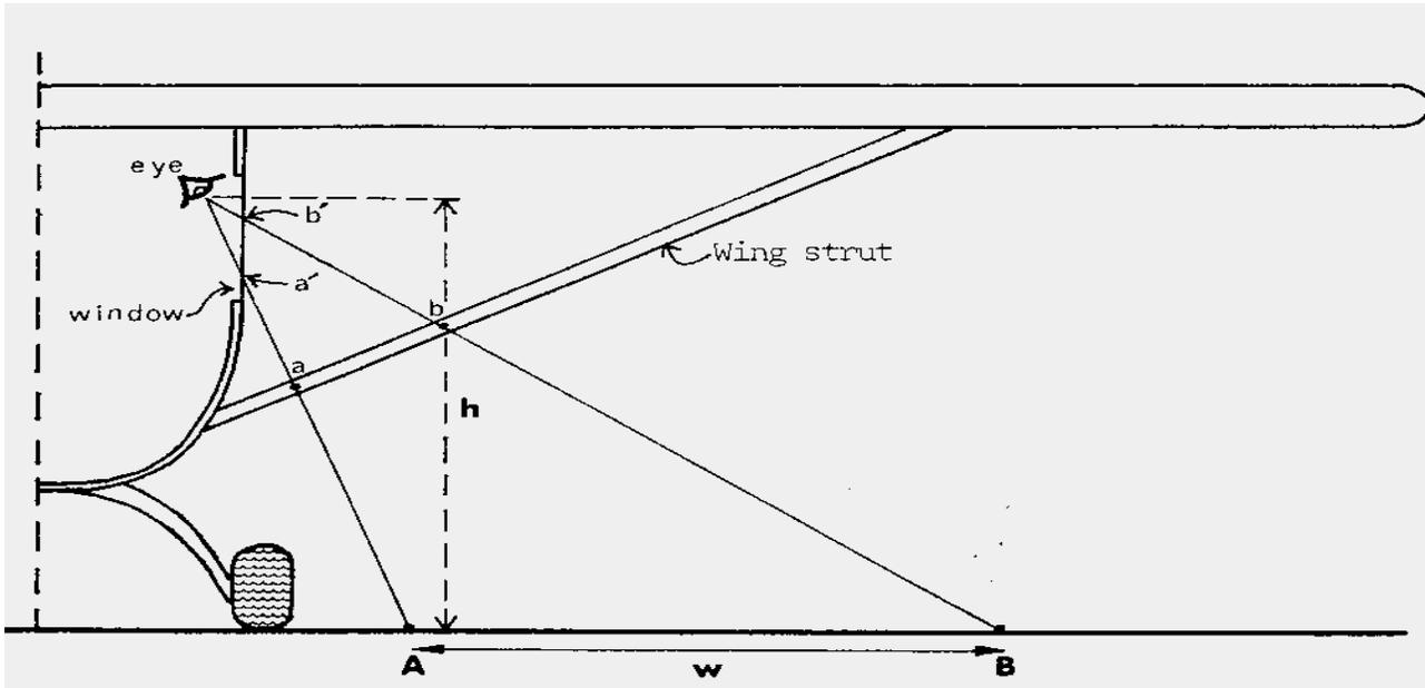
Figure 7. Schematic diagram of aircraft configuration for strip width sampling (Norton-Griffiths, 1978).  $W$  is marked out on the tarmac, and the two lines of sight  $a' - a - A$  and  $b' - b - B$  established. The streamers are attached to the struts at  $a$  and  $b$ , whereas  $a'$  and  $b'$  are the window marks.
