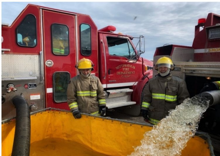
Pictured Left: A Fire Department Pump Operator demonstrating drafting techniques to effectively supply the fire truck with water.
