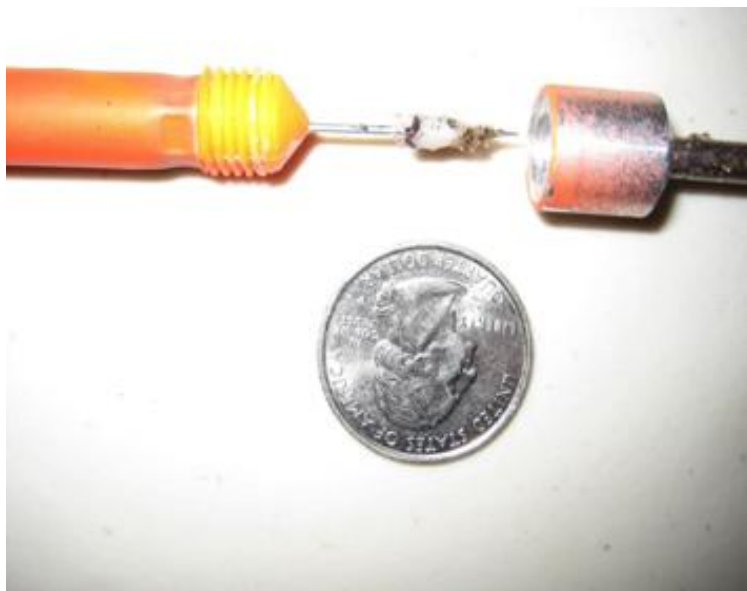
Figure 5. Example of a disassembled biopsy dart tip showing the extracted skin sample during the sampling process.
