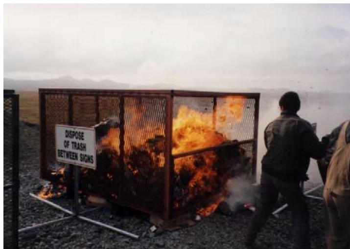
Figure 3 – Open Metal Burn Box Photo courtesy of Alaska Department of Environmental Conservation
